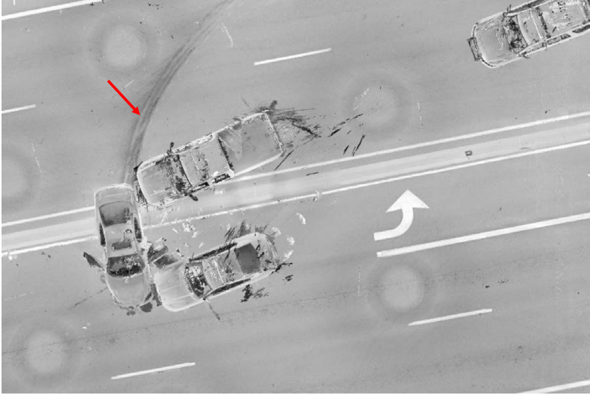
A closer view of the crash. The red arrow identifies markings on the road following Lee's course of travel, showing a path from the brick wall on the north side of McCarran.
